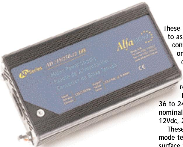
These power supplies, commonly referred to as 'brick in the lead' units, offer a convenient way to use 12Vdc, 24Vdc or 48Vdc equipment from alternating current supplies of between 85 to 135Vac and 170 to 265Vac. Input voltage selection is automatic and requires no manual adjustment.
